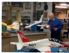
Tom Reinbolt's show and tell was another Freewing model of the L-39 Albatros. Wingspan is 41.5 inches and the length is 53 inches. It uses a 80mm twelve blade fan powered by a six cell lipo and 100 amp speed contoller. Tom used Orange-Glo on his model too. BJ
