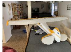
Yours truly brought his Premier Cessna 170. Wing span is 86 inches. It weighs nine pounds and can be powered with a four, five or six cell lipo battery. Prop is 16 inches. No Orange-Glo yet. BJ
